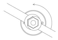
2) Secure the End Fitting with a second wrench and rotate it counter-clockwise several turns until it is free.
